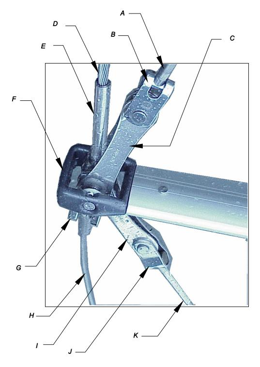
G H D2 stem T jaw toggle V1 Α В jaw toggle link plates С link plates jaw toggle D **V**2 RD1 stem T K marine eye E F spreader tip casting
