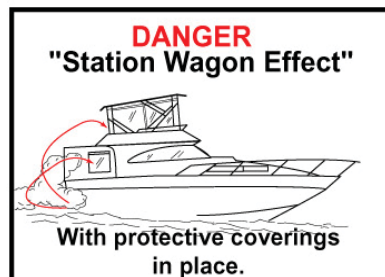
Figure 4.6. When protective weather coverings are in place, engine or generator exhaust from your boat, while docked and/or running, can cause excessive accumulation of Carbon Monoxide gas within the cabin and cockpit areas of your boat. Always provide adequate ventilation when the weather coverings are in place and either the engine or generator are running.
