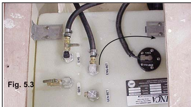
In Fig.5.3 you can see the fuel supply fittings. The photo inset shows the close-up of the fuel valve. See Fig.5.5 for the function of the fuel valves.
