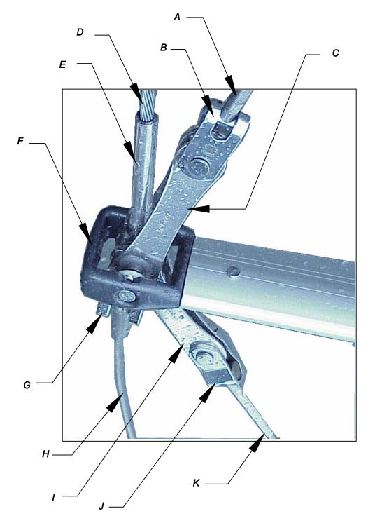
D2 stem T jaw toggle V1 G H Α jaw toggle B C D link plates link plates V2 jaw toggle RD1 stem T E F Κ marine eye spreader tip casting
