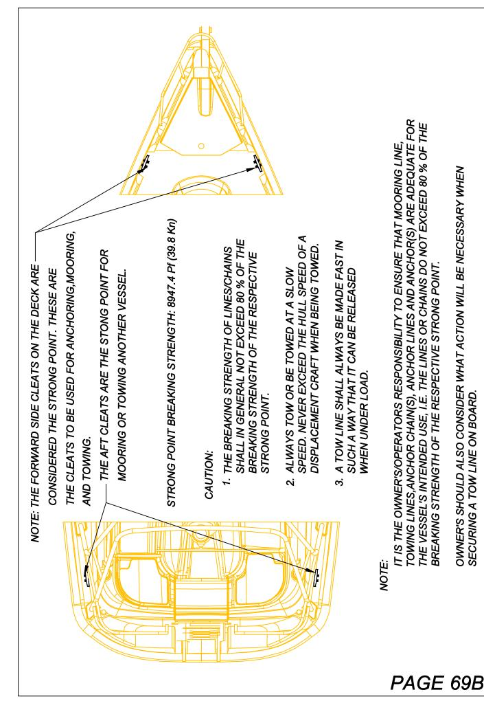
THE VESSEL'S INTENDED USE, I.E. THE LINES OR CHAINS DO NOT EXCEED 80 % OF THE BREAKING STRENGTH OF THE RESPECTIVE STRONG POINT. **OWNER'S SHOULD ALSO CONSIDER WHAT ACTION WILL BE NECESSARY WHEN** SECURING A TOW LINE ON BOARD.
