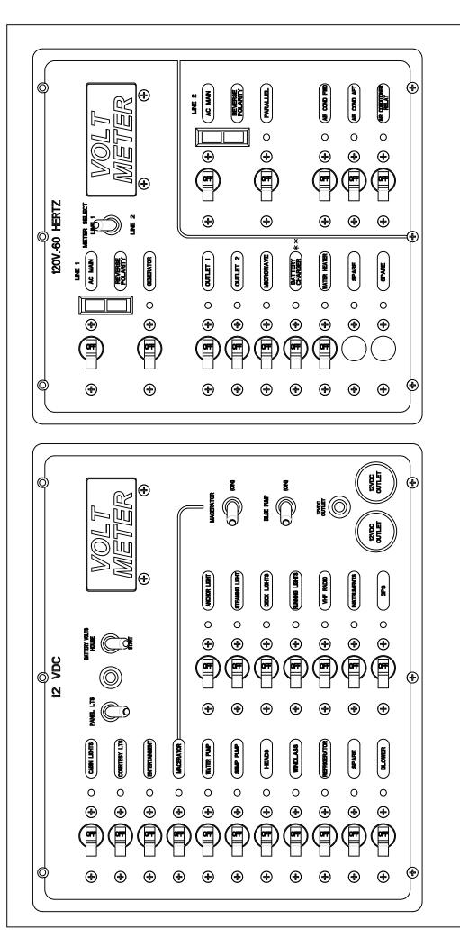
\*\*IF THE BOAT IS EQUIPPED WITH AN INVERTER INSTEAD OF BATTERY CHARGER, THIS BREAKER BECOMES A SPARE. POSSIBLE CONFIGURATIONS FOR THE SPARES ON THIS PANEL MAY INCLUDE THE WASHER/DRYER, WATERMAKER, OR ICEMAKER OPTIONS. This document discloses information for which HUNTER NARNE CORP. has proprietary rights
