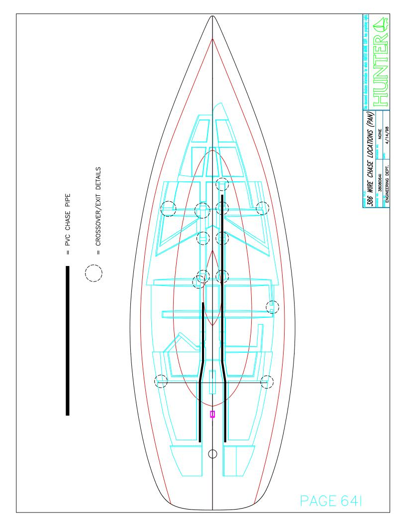
This document discloses information for which HUNTER NARNE CORP. has proprietary right THIS PAGE IS PROVIDED FOR ANY ADDITIONAL DC ELECTRICAL INFORMATION. 386 DC CONSUMER NOTES 1. ALL DC WIRING WITHIN 12" OF ANY COMPASS SHALL BE TWISTED PAIRS ... THAT IS THE HOT LINE AND GROUND SHALL BE TWISTED TOGETHER. ENGINEERING DEPT. 3808064J PAGE 64J
