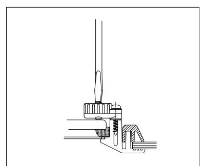
Periaodic adjustment of the dog might be necessary to maintain proper pressure. This is accomplished by turning the set screw at the tip of the dog clockwise while the dog is disengaged. Turn the set screw half a turn and check for proper compression of the gasket. Do not over tighten.
