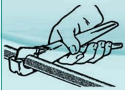
Cut the tubing to length using the Sea Tech tubing cutter or similar. Inspect the outside diameter of the tubing. It must be free of damage, smooth, and clean.
