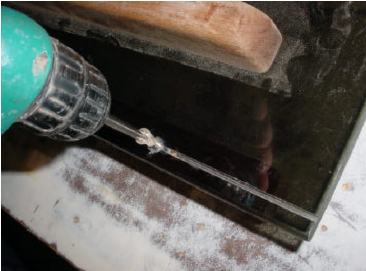
Fig 4. Use 4 pieces #10 x 1-1/4" long flat head wood screws to hold top pull to plexiglass
