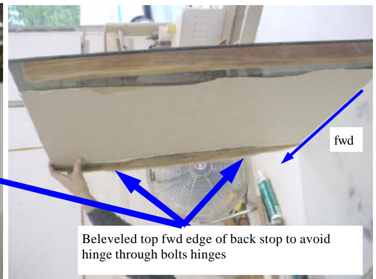
Fig 5. Side view of installation complete top teak pull and bottom pull
