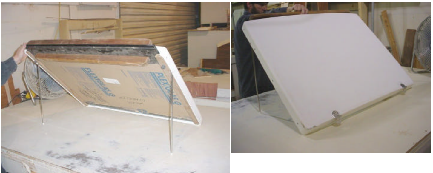
Fig 9. Sea hood assembly Installation complete
