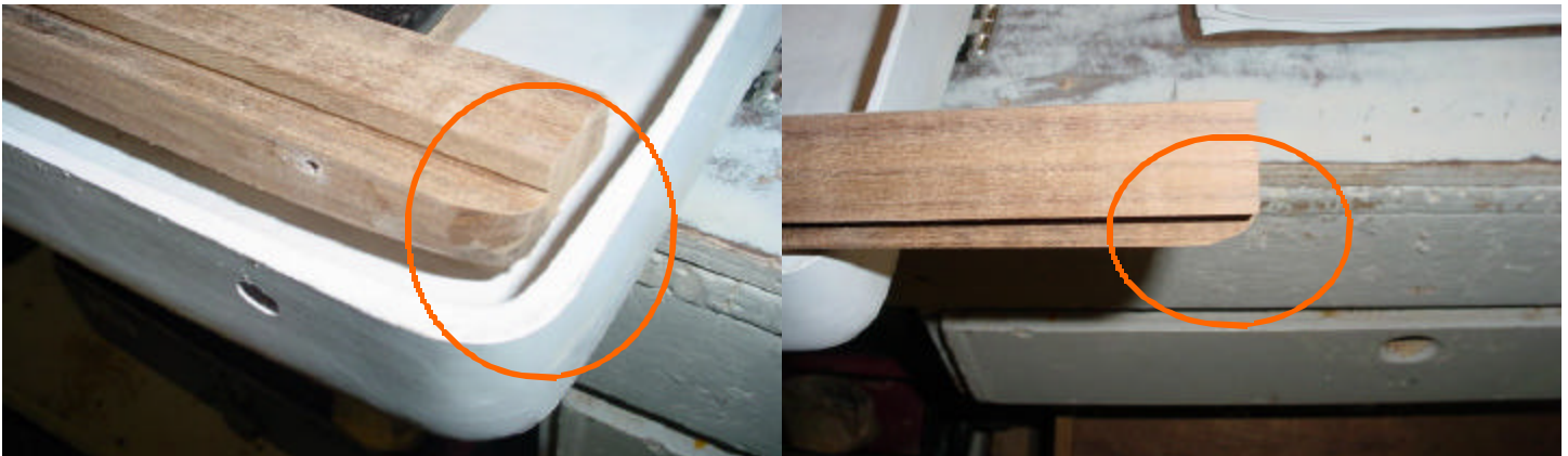
Fig 2. Sanding fwd edge of teak track in order to fit fwd inside corner of fiberglass sea hood. Sanding aft edge of teak track in order to fit aft inside corner of fiberglass sea hood. Do the same procedure to the other teak sliding track.
