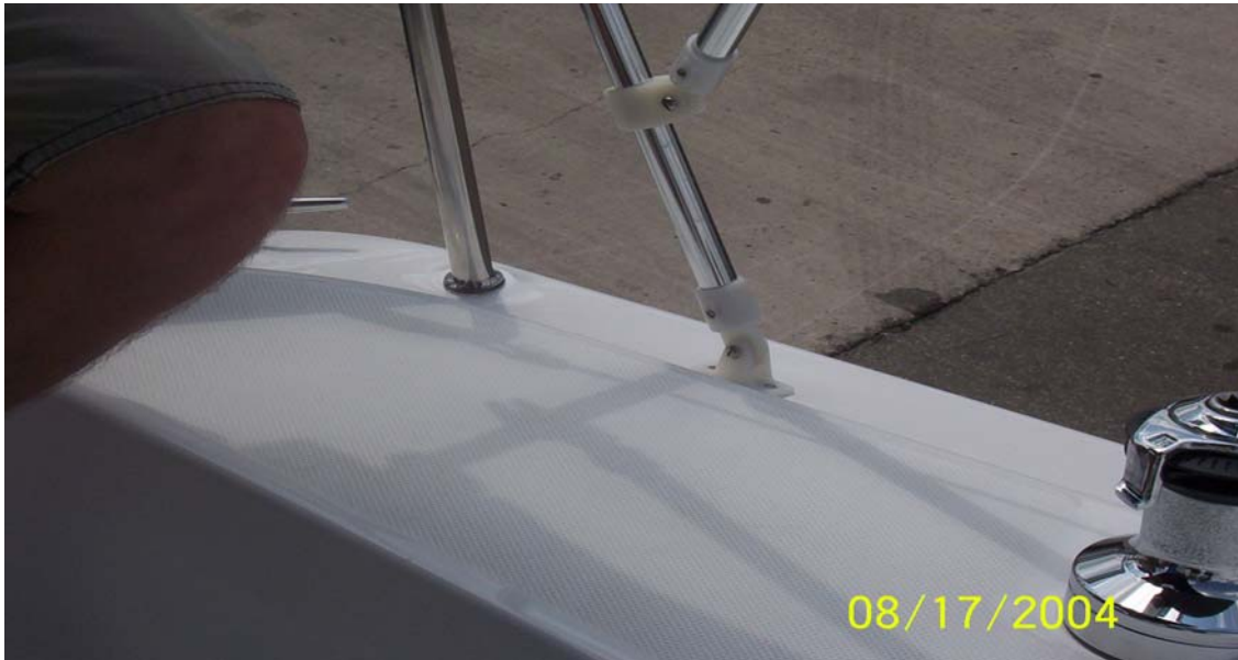
(Picture #1) Measure 9" fwd to find center of mount
