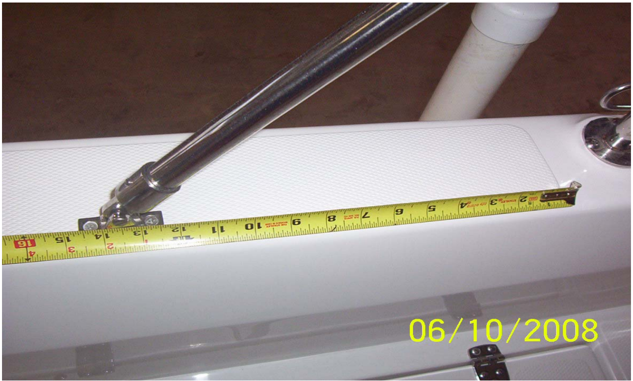
(Picture #1) Measure 13" fwd to find center of mount
