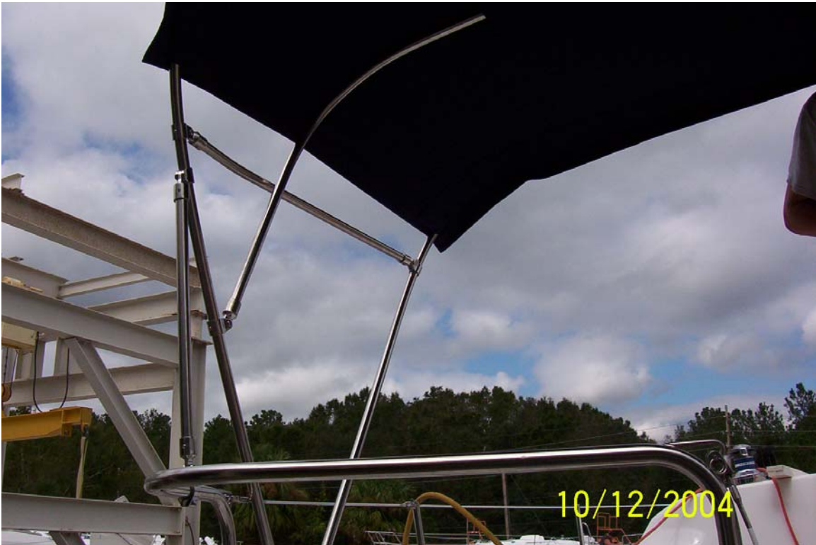
(Picture #3) Attach the smaller stiff leg
