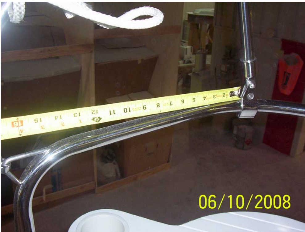
STIFF LEG MOUNTS 16" AFT OF STERN RAIL
