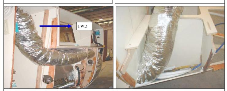
Run air duct thru galley divider bulkhead cutout to aft cabin starboard side hanging locker, install round air vent on hanging locker aft face cutout then install Air duct on air vent
