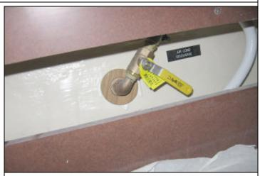
Install AC discharge thru hull fitting, wood doughnut, ball valve and the ball valve handle facing 4:30 direction as you facing starboard side, install the other end of discharge hose to this thru hull and secure the hose using 2 designated hose clamps
