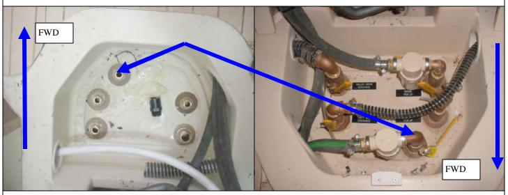
Air conditioning water pick up thru hull fitting, drill  $\emptyset$ 1-1/8" bilge thru hull hole at indicated location for air conditioning pick up fitting, ball valve. Illustration at right shown view of complete air conditioning pick up thru hull's installation.
