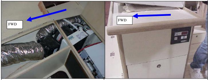
View of air conditioner unit is installed inside starboard side bunk. Air duct runs forward to V berth starboard side and the other air duct runs afterward to QB hanging locker aft face. View of air conditioner unit electronic control unit is mounted on galley inboard face aft corner.
