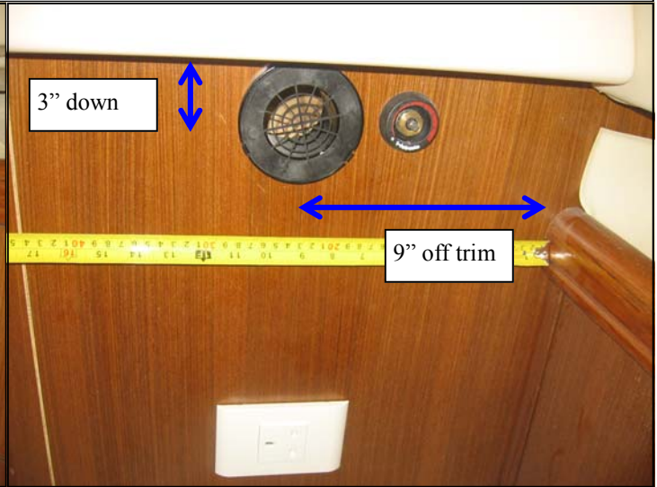
Inlet air nozzle locate 3" down glass headliner and 9" off teak trim
