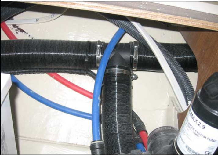
Air duct comes from heater unit, under galley then to port bunk. Install T junction at this location.
