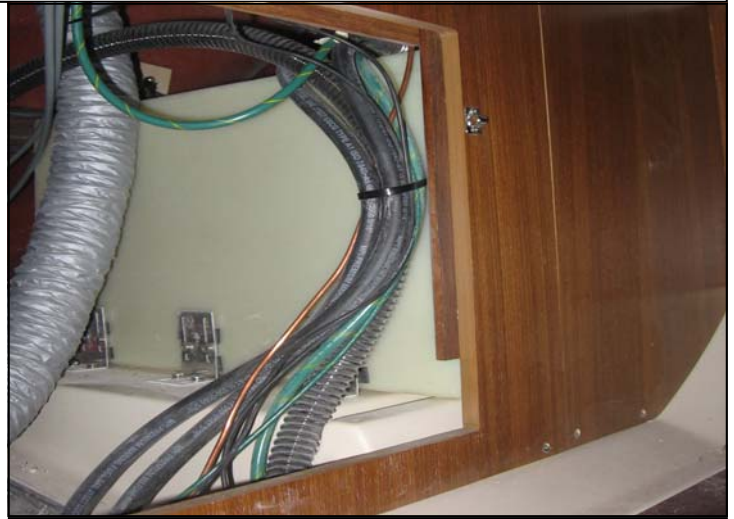
Copper fuel line runs along with engine fuel line under aft bunk.
