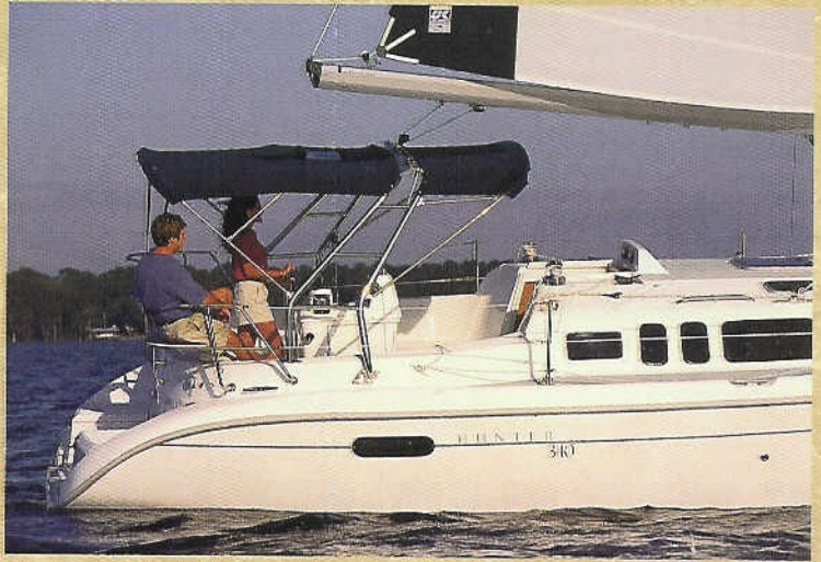
The integrated arch keeps the cockpit clear with the traveler up top and makes a great attachment point for the optional bimini.
