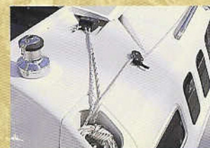
All lines are led aft for short-handed sailing and the coaming walls keep it all organized.
