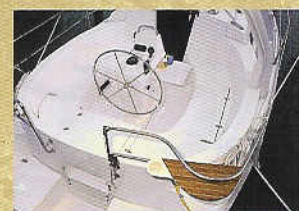
The rounded cockpit is pushed right to the gunnels to provide maximum useable space.
