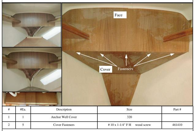
Note: The face for the cover is installed in the Pre-deck stage.
