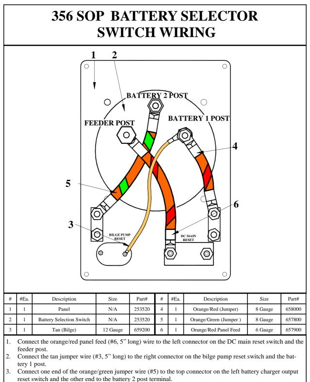
4. Connect one end of the orange/red jumper wire (#4) to the top connector on the right battery charger output reset switch and the other end to the battery 1 post terminal.
