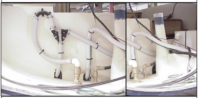
NOTE: All hoses will be connected with two clamps on both ends of the hoses or Valve
