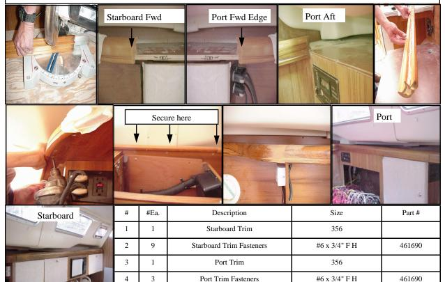
1. The <u>starboard trim</u> is located on the upper inboard starboard shelf of the main cabin. The aft end will be flush with the aft galley bulkhead wall.
