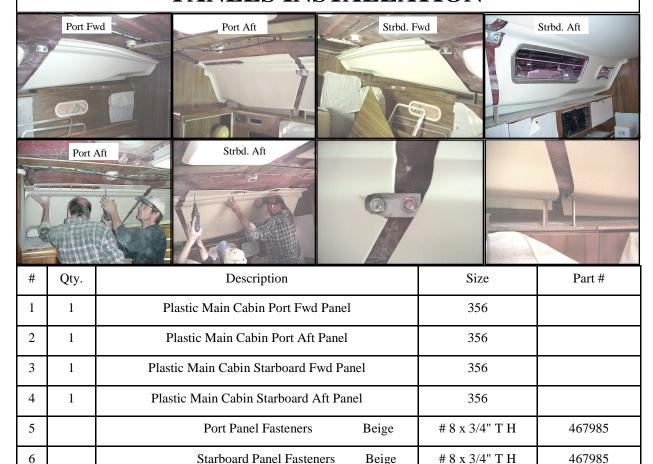
There are four plastic headliner panels in the Main Cabin, one port fwd, one port aft, one starboard fwd, and one starboard aft.
