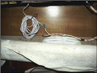
CUT OFF THE ENDS OF ALL WIRES AND EXCESS SPEAKER WIRE GOING TO SPEAKER
