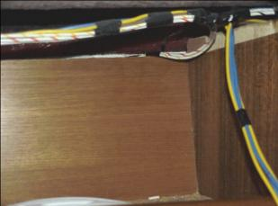
TUCK WIRES BACK BEHIND HULL PANEL
