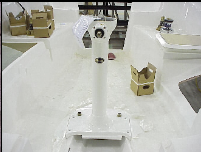
PEDESTAL IN EMBOSSMENT, MAKE SURE PEDESTAL IS SLID ALL THE WAY FORWARD THEM MARK MOUNTING HOLE LOCATIONS
