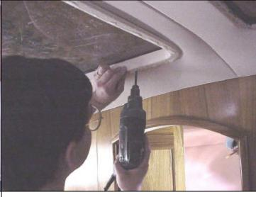
Secure ring in place using #8 x 3/4" beige truss head screws.
