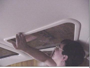
Check trim rings for fit, there should be a 1/8" gap between the top of the ring & the windshield.
