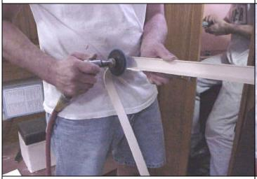
Grind down top of ring if necessary to obtain proper gap. Deburr ring after trimming.
