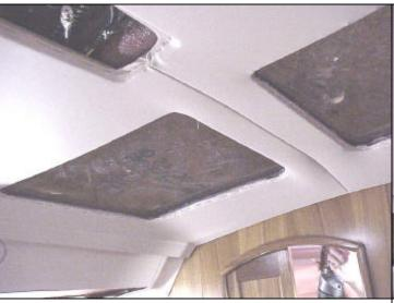
Headliner ready for trim rings. Whisper is stapled to the inside of the wood not the bottom.
