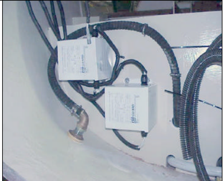
Generator exhaust thru hull assembly is mounted port side aft hull, the assembly contains \phi 1-1/2 " chrome thru hull fitting, brass elbow with 1.5" FPT x 1.5" barb. The thru hull diameter is 2".
