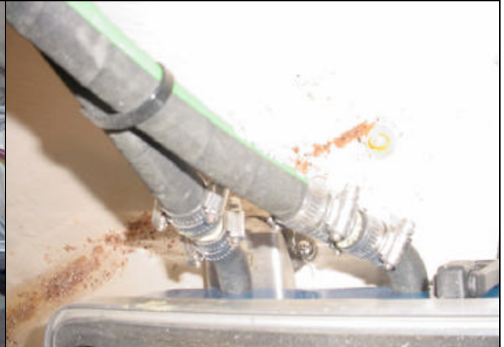
Fig 2. Install fittings & coolant hoses ( 23.6" long), secure hoses using designated hose clamps.
