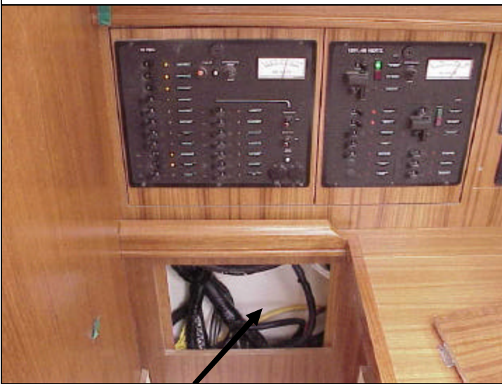
The auto pilot wires should be in the harness under the AC & DC panels. They will have the same numbers, wire size, & color as the wires in the back.
