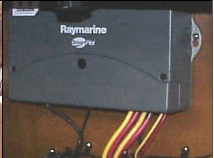
Photo of the compass computer after the face has been removed from the forward end of the nav station.
