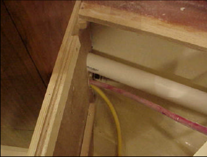
1/0 Cables going from bow thruster motor to port side of boat & aft thru hanging locker.
