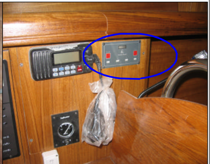
Mount the remote control panel next to VHF radio
