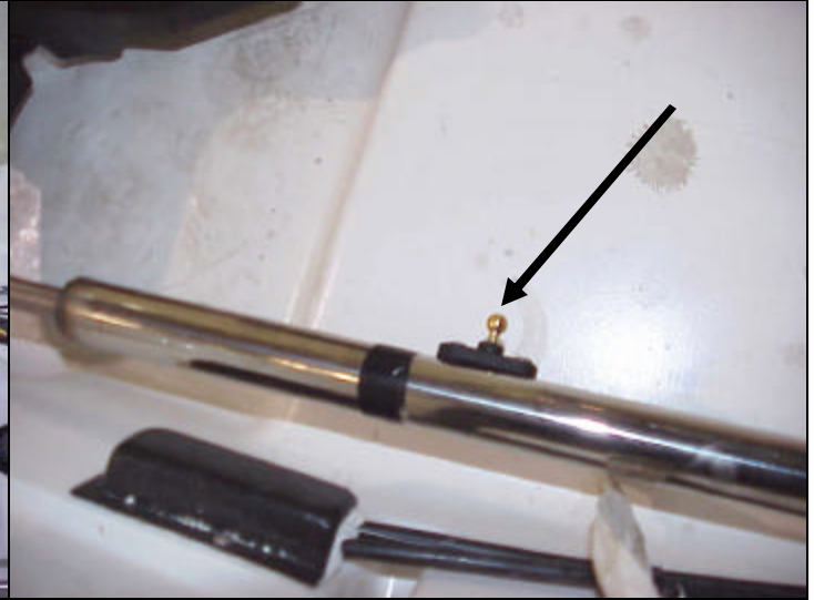
Pivot ball of rudder reference sensor unit connected to steering drag link (drill and tap drag link). Put tape on the drag link to show where rudder steering arm hits drag link, pivot ball for rudder reference unit must be forward of the tape.
