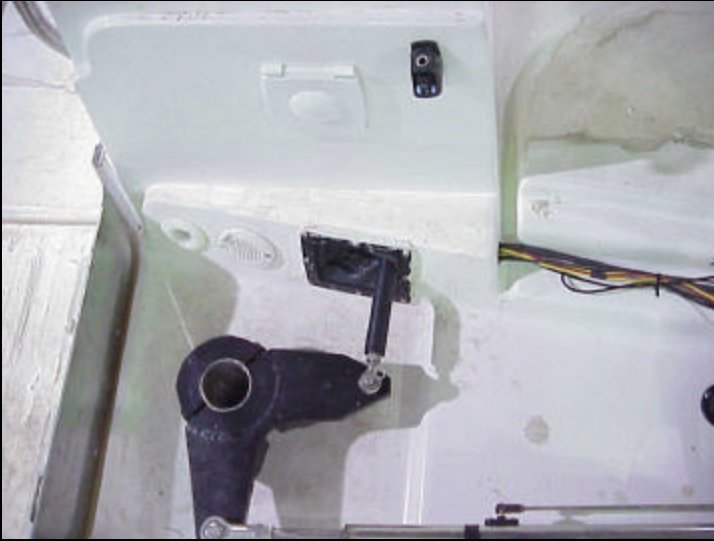
Drive unit arm attached to rudder steering arm. NOTE: Seal boot coming thru deck well with caulk.
