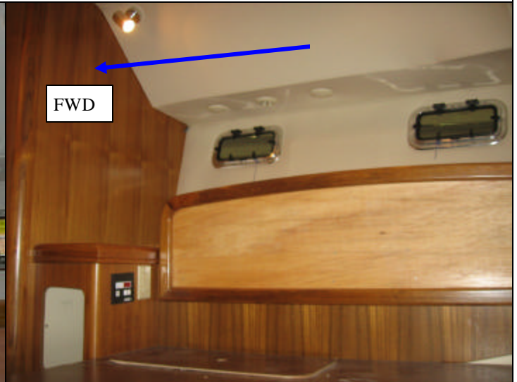
Aft Cabin Starboard Side Air Vents (3 vents)
