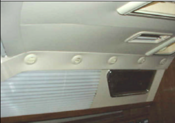
Main Cabin Starboard Side Air Vents (5 Vents)
