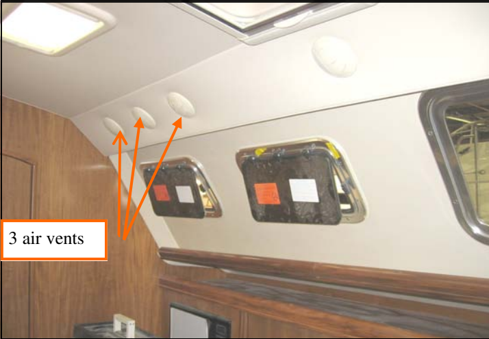
3 air vents locate above main cabin port side aft portlight area.
