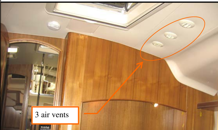
3 air vents locate on port side headliner in fwd cabin.
