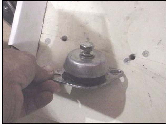
One of the four feet that come with the generator. The bolt in the top is metric so don't lose it.
