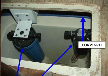
FILTER & BOOSTER PUMP MOUNTED IN BILGE COM-PARTMENT JUST FORWARD OF THE AFT-INBOARD CORNER OF THE PORT BUNK TUBE FROM PICKUP THRU HULL GOES TO "IN" SIDE OF BOOSTER PUMP. THEN CONNECT "OUT" SIDE OF PUMP TO "IN" SIDE OF FILTER. "OUT" SIDE OF FILTER WILL BE PLUMBED TO "IN" SIDE OF HIGH PRESSURE PUMP ON THE WATER-MAKER.
