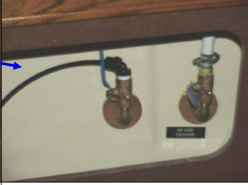
DISCHARGE THRU HULL IN FORWARD SECTION OF PORT BUNK BACKREST. HANDLE ON AFT SIDE OF BALL VALVE & POINTS UP WHEN CLOSED. OTHER END OF TUBE CONNECTED TO "BRINE OUT" ON WATERMAKER MANIFOLD.
