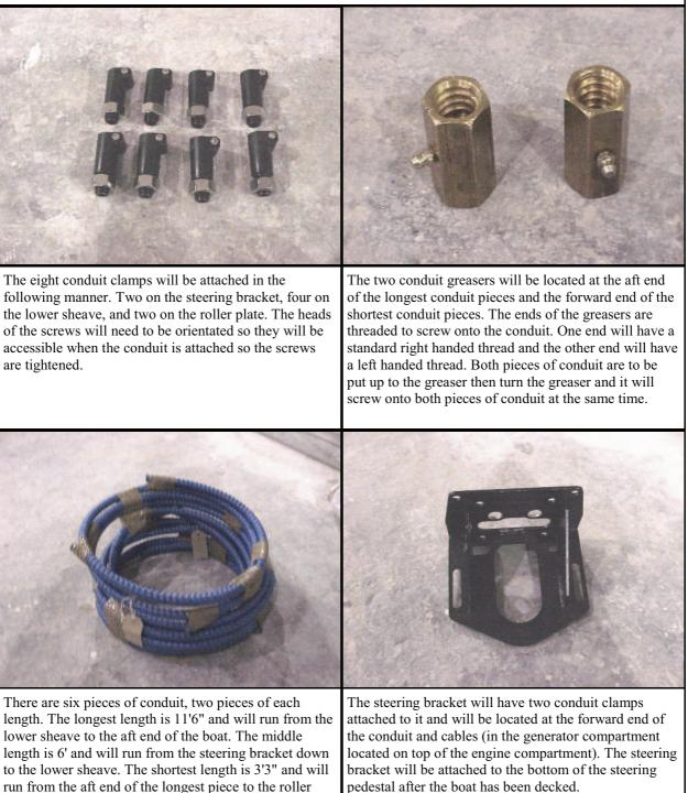
plate. A conduit greaser will be installed between (and connect) the longest piece and the shortest piece of
