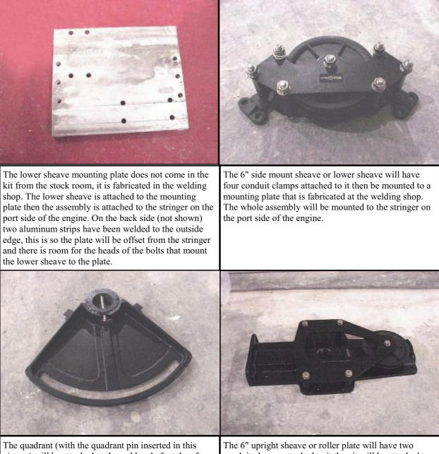
The quadrant (with the quadrant pin inserted in this picture) will be attached to the rudder shaft at the aft end of the boat. The steering cables will be attached to the quadrant via the eye-bolts and u-bolt style cable clips.
