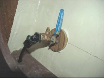
DISCHARGE THRU HULL IN AFT SECTION OF PORT BUNK BACKREST. HANDLE ON FORWARD SIDE OF BALL VALVE & POINTS INBOARD WHEN CLOSED. OTHER END OF TUBE CONNECTED TO "BRINE OUT" ON WATERMAKER MANIFOLD.
