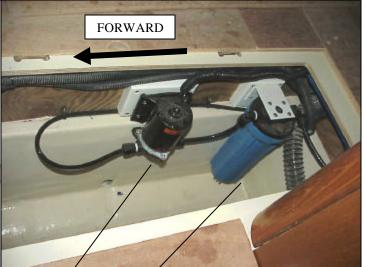
BOOSTER PUMP & FILTER MOUNTED IN BILGE COM-PARTMENT JUST INBOARD OF WATERMAKER TUBE FROM PICKUP THRU HULL GOES TO "IN" SIDE OF BOOSTER PUMP. THEN CONNECT "OUT" SIDE OF PUMP TO "IN" SIDE OF FILTER. "OUT" SIDE OF FILTER WILL BE PLUMBED TO "IN" SIDE OF HIGH PRESSURE PUMP ON THE WATERMAKER.
