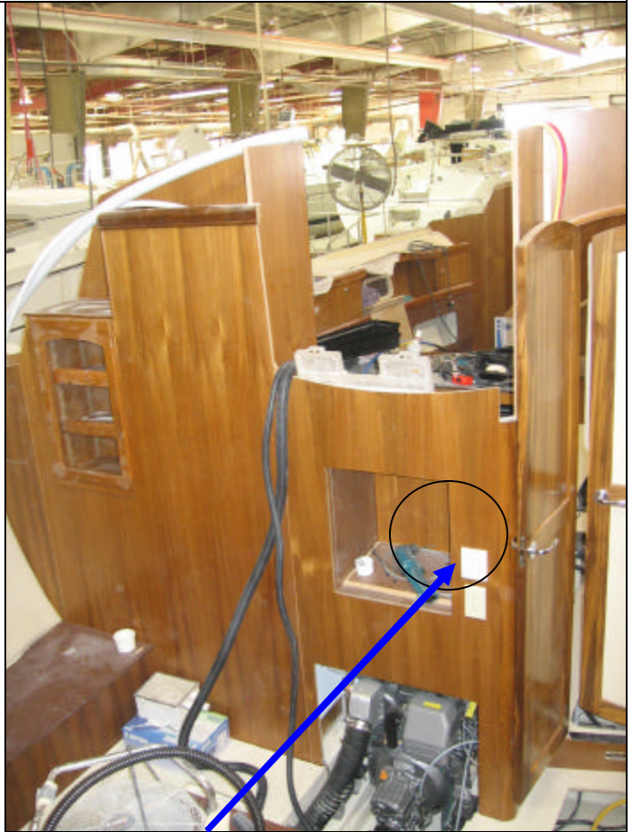
Aft air conditioner ECU will be installed on aft engine cabinet if the boat gets air conditioner option
