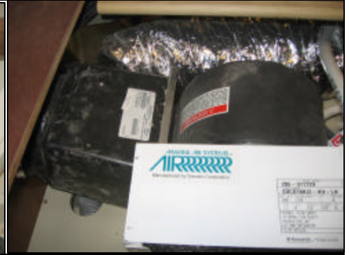
Install all air ducts at bunk side to air duct distribution box.
