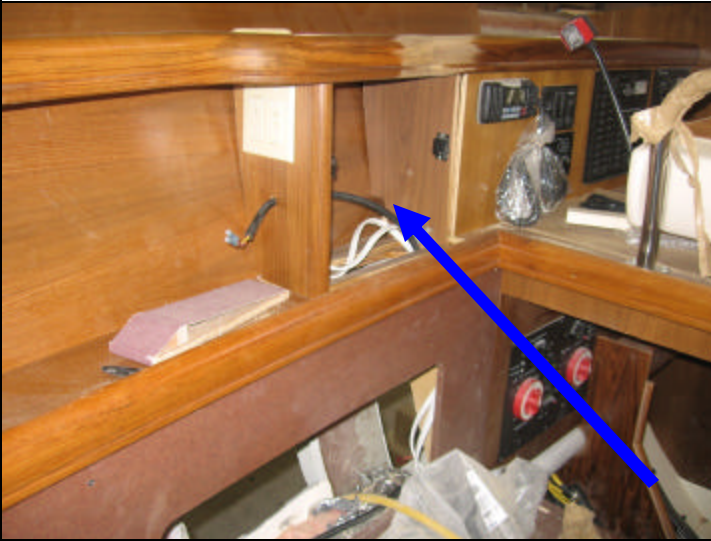
Air duct and ECU for fwd Air conditioner unit will be installed in this shelf
