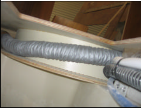
Air duct runs along toe kick radius in main bilge fwd compartment of the pan
