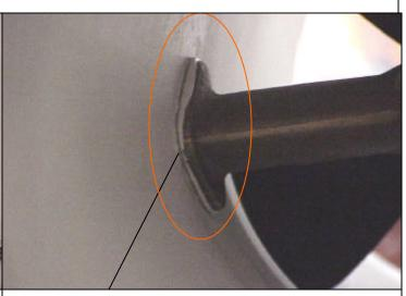
Apply qualified marine sealant 5200 to caulk around gear unit mounting hole.
