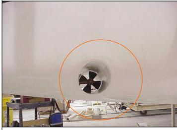
Bow Thruster duct inlet radius, patching port & starboard side radius to 10~15% of bow thruster tube diameter. \*\*\*
