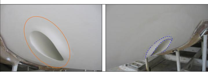
The radius of this lip is essential, the radius should be 10-15% of bow thruster tube diameter.
