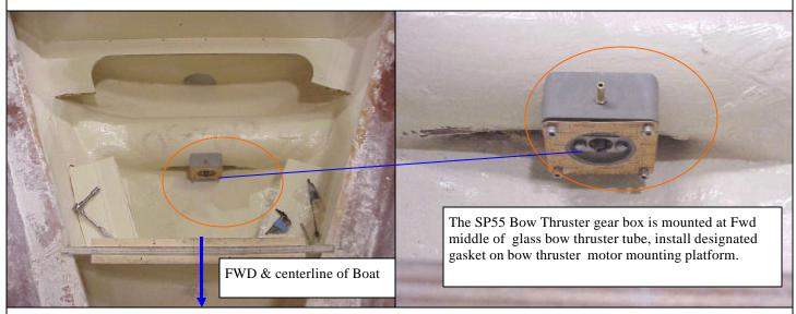
Interior Gel-coat is applied after the bow thruster tube is boned & scuffing. Locate gear box mounting hole after gel-coat is cured.
