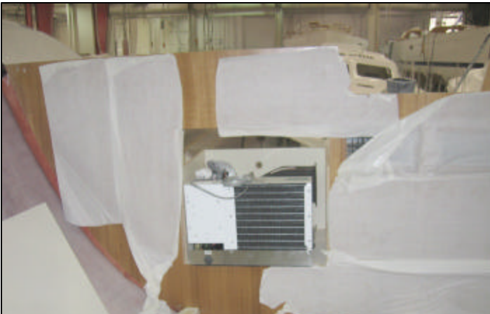
Place Air conditioner unit in A/C shelf, the shelf is aft kick-board bulkhead starboard side. The platform is bonded to hull. Bonding material is gel coated.
