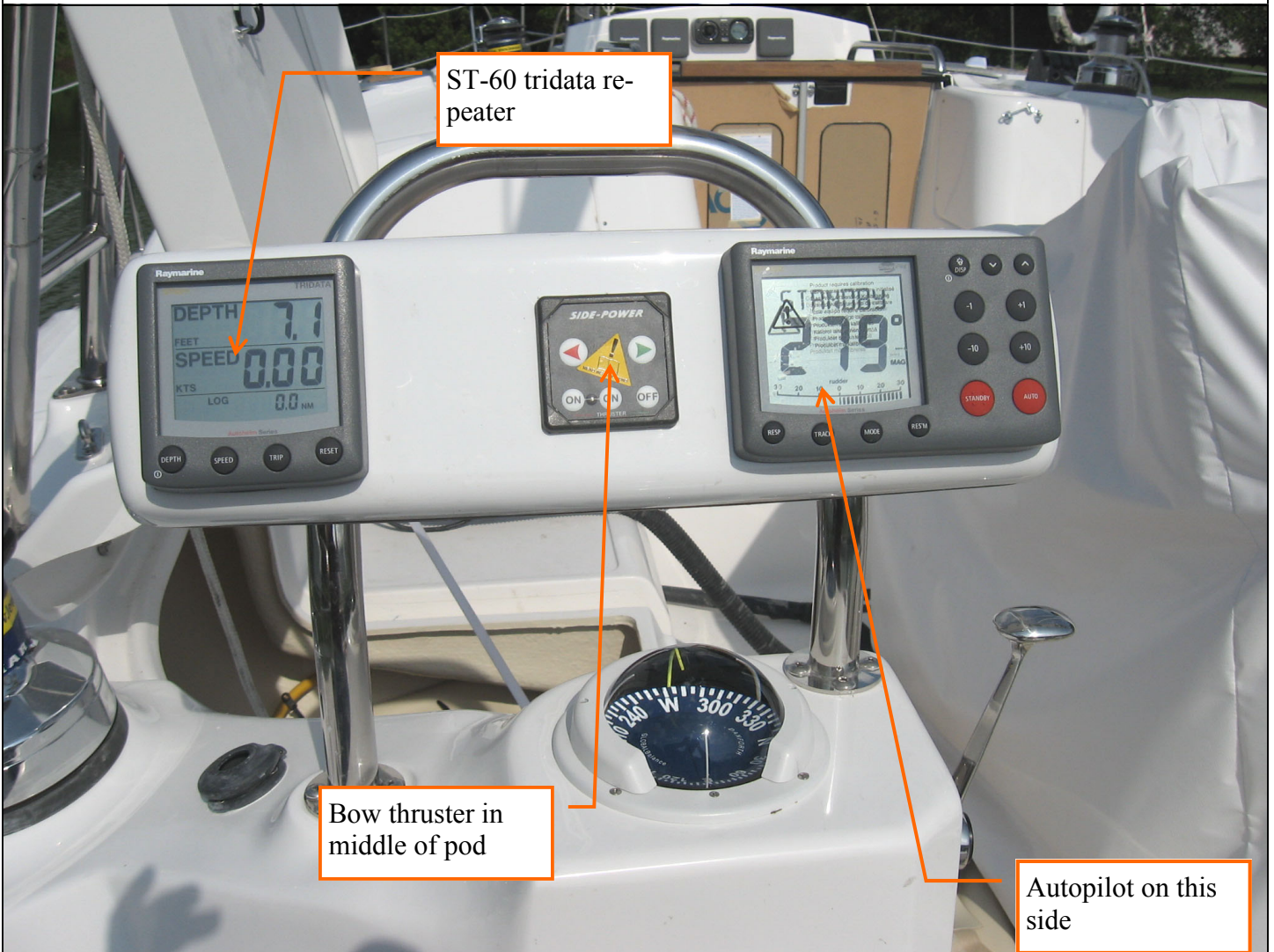
Cockpit port helm station NAV pod
