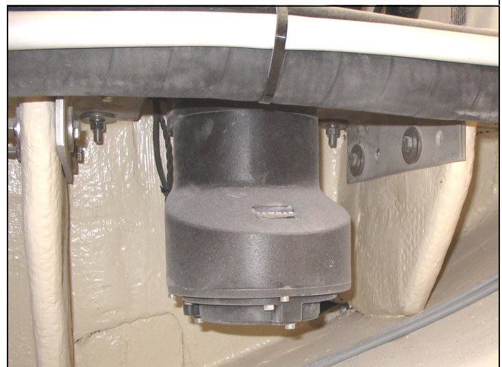
Autopilot drive unit under starboard side steering drive
