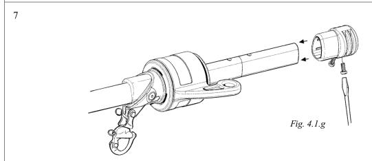
Fit the halyard swivel over the top end of the extrusion, slide it down as far as the sail feeder and secure it in this position with adhesive tape. Fit the top guard and secure it with the two pre-fitted screws. Tighten the screws until they bottom, but do not over-tighten.
