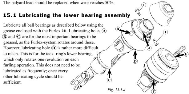
**Tools**: 1 Torx spanner or screwdriver. (The Torx spanner set supplied with the Furlex-system is suitable.) 1 pair of long-nosed pliers
