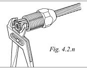
12. Insert the former into the threaded hole of the terminal part (or rigging screw). Lubricate the socket's thread with a long bead of locking adhesive. Screw the terminal part onto the socket and tighten carefully, forcing the wire further into the terminal.
