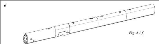
Connect the remaining extrusions according to "Table 2" (3.6.1).
