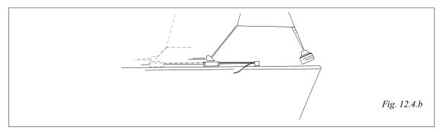
Many furling foresails have markings in the foot for different reefing positions. After you have tested combinations of sail area and sheeting position to see which function satisfactorily, you can use these markings as a reference and mark suitable sheet points on the track.
