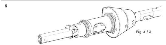
Feed the adapter on to the adapter tube, cover the tube with some kind of protection and secure it to the luff section with adhesive tape.
