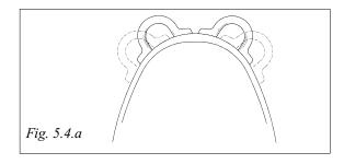
To avoid corrosion between the bronze lead and the aluminium mast, each lead is supplied with a self-adhesive insulator sheet. It is important to fit this between the lead and the mast.
