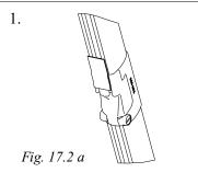
Secure the stainless steel sail feeder with adhesive tape to prevent it from falling overboard during disassembly.
