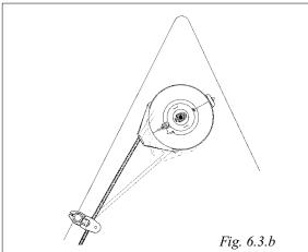
Slacken the locking screw ③ a little. (See Fig. 4.3.f.) Align the eye of the line guide to the first lead block as shown in the diagram above. Tighten the locking screw.
