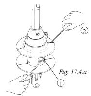
Insert a screwdriver ① under one of the connecting clips. At the same time, press another screwdriver ② between the drum halves on the same side so that these are forced apart 3–4 mm.
