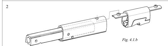
Fit the long connecting plate at the same time as the sail feeder as shown in the diagram. Push the joining sleeve up so that it is flush with the top edge of the sail feeder.
