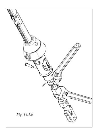
6. Place one wrench over the flat faces of the wire terminal and the other over the flat faces of the rigging screw body. Adjust the position of the rigging screw by turning the **body of the rigging screw** until the desired forestay length is obtained. **Note! Do not turn the wire terminal.**
