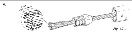
Slide the wedge over the core (7 strands) of the wire. The core of the wire should protrude approx.  $2 \text{ mm} (3/32^{\circ})$  from the wedge.
