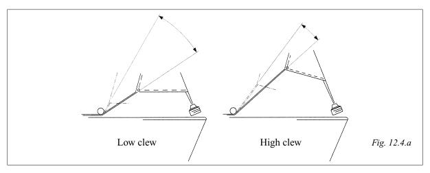
The angular variation of the sheet relative to the deck is less for a high-clewed sail. The comparison is based on the same number of furling revolutions.
