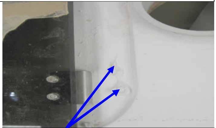
Caulk around on fwd-stop mounting holes, 2 mounting holes on each side
