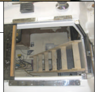
Install slider stainless plate on inboard raised embossment
