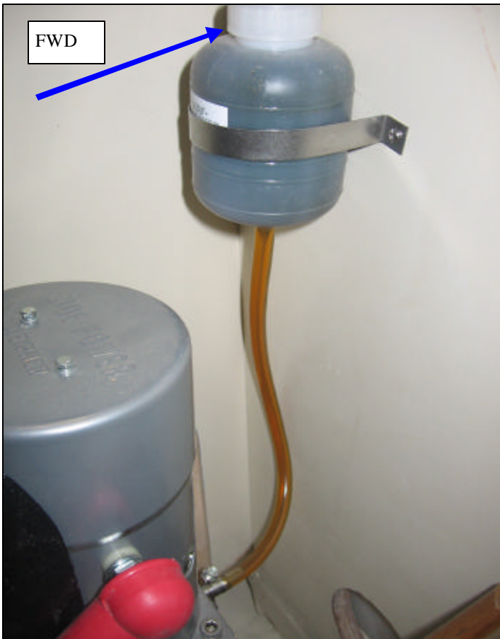
Overview of bow thruster drive unit installation, oil reservoir bottle is mounted fwd upper of drive unit
