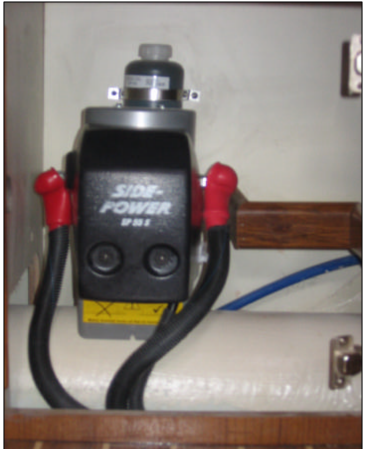
Overview of bow thruster drive unit installation, oil reservoir bottle is mounted fwd upper of drive unit
