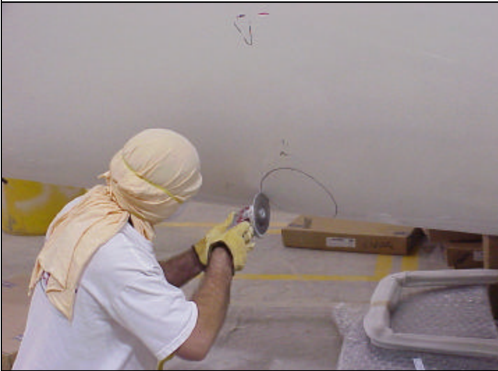
Mark & cutout hull to receive bow thruster tube.
