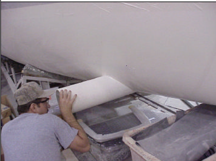
Insert bow thruster tube.
