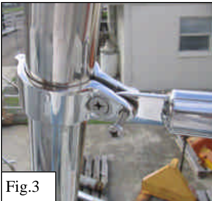
Strut & jaw slide, the slide is mounted to CA and strut is installed to jaw
