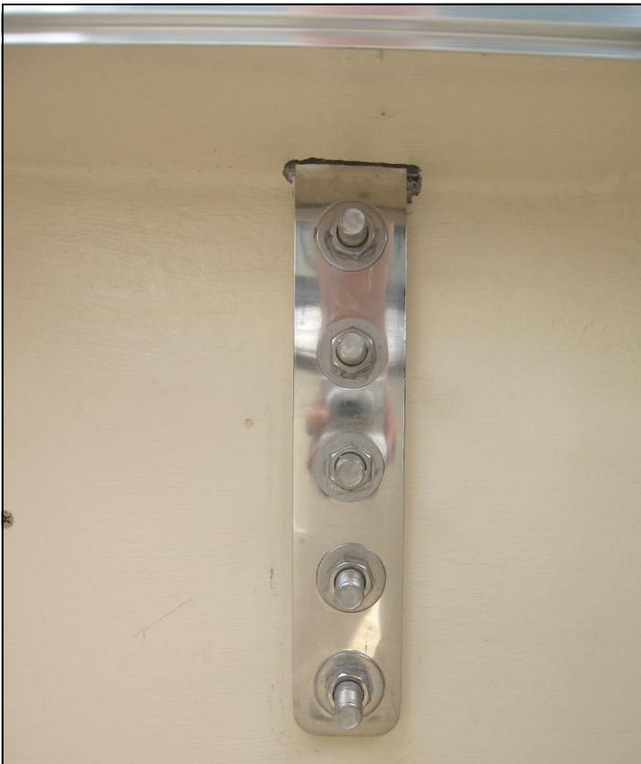
The picture shows the installation of the chainplate in sail locker aft bulkhead.
