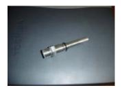
6) Use the Petroleum Jelly provided to grease the aluminum pin. Place the small rubber O-ring in the thin slot machined in the pin and grease it as well.
