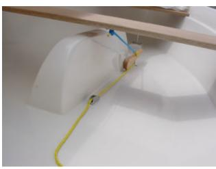
Mount the clam cleat on the floor 3" forward of the aft end of the centerboard trunk, inline with the handle (approx. 1" from the centerboard trunk). Use the screws provided and DO NOT drill pilot holes for the screws.
