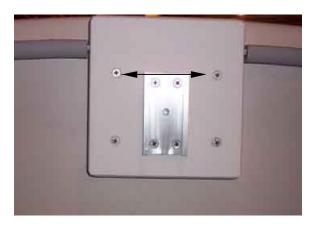
10) Mount the aluminum receiver bracket (with the open side up!) for the rudder gudgeon using the 4-#10 x ¾" flat head tapping screws. Position it in the center of the transom block with the top aligned with the top 2 screws that hold the block to the boat. Drill pilot holes for the screws and mark and drill a clearance hole in the center for the thumbscrew. Note: You may have the wooden transom block-the alignment is the same.
