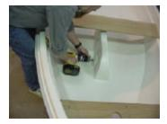
4) Remove the nylon disc from the starboard side of the centerboard trunk. Remove the old sealant.
