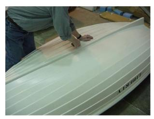
another thin piece of plywood depending on when your boat was manufactured). Stab the plywood with the razor and remove and discard (also the thin piece if it is present). Inspect the centerboard trunk and make sure that it is clear. There may be a piece of tape holding the centerboard pin bearing, which is supposed to be there. Dry fit the centerboard to insure proper clearance.
