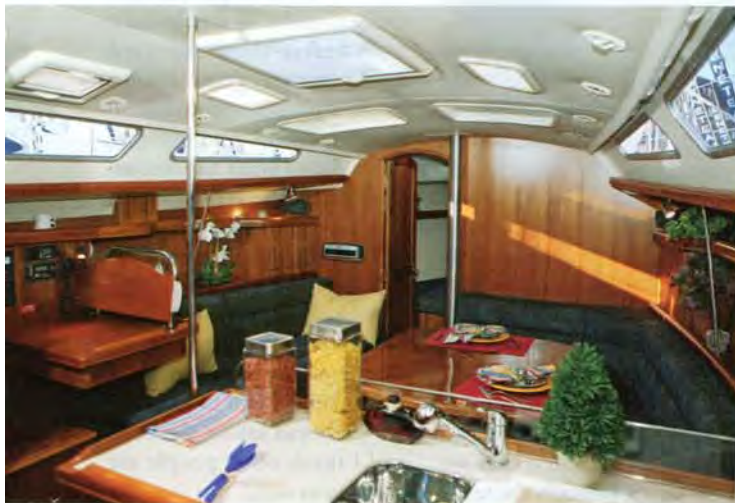
With stainless-steel tie-rods and posts supporting the rig and deck—and with plenty of portlights and hatches in the overhead—the Hunter's interior is especially light and open.
