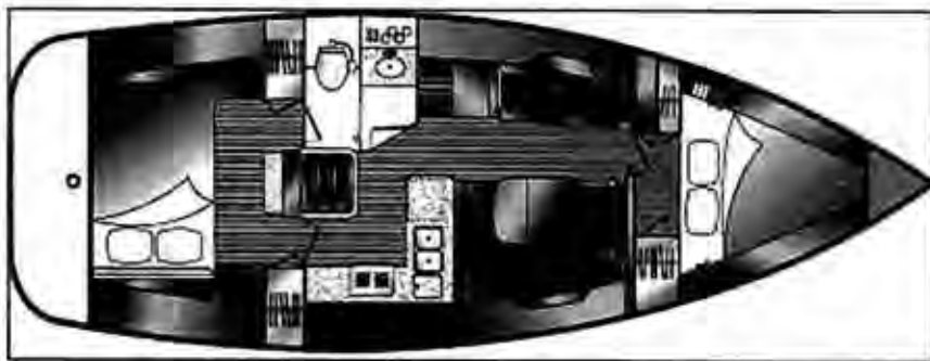
Hunter packs a lot into the 38's interior. The boat is offered in both the two-cabin layout shown here, and a three-cabin version.
