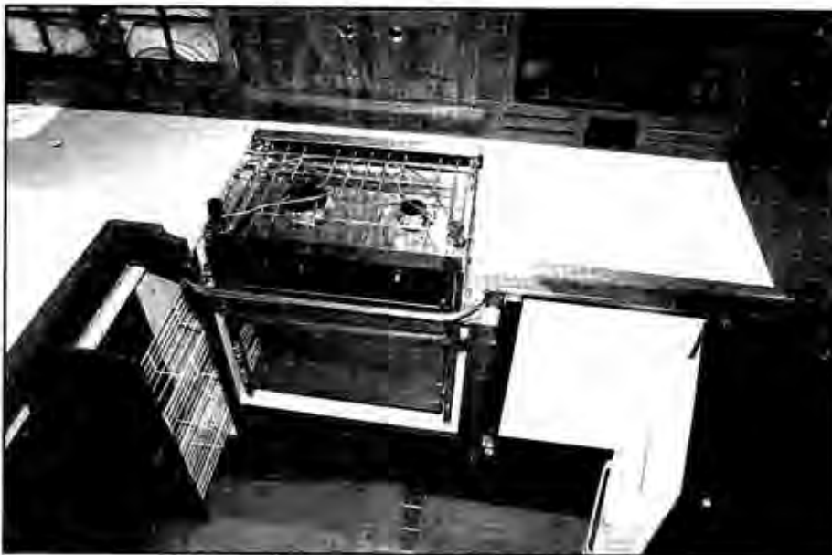
The Hunter 38's galley has enough surface area for food preparation, plus stowage for both food and cooking gear. We like the stout fiddles, but would prefer something less heavy than Corian for countertops. The stove/oven combo is standard, but refrigerator and microwave are optional.
