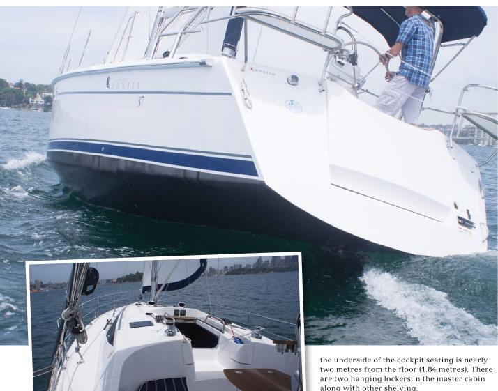
MAIN: Underbody with the beamy flat aft sections clearly defined by the waterline chine.
