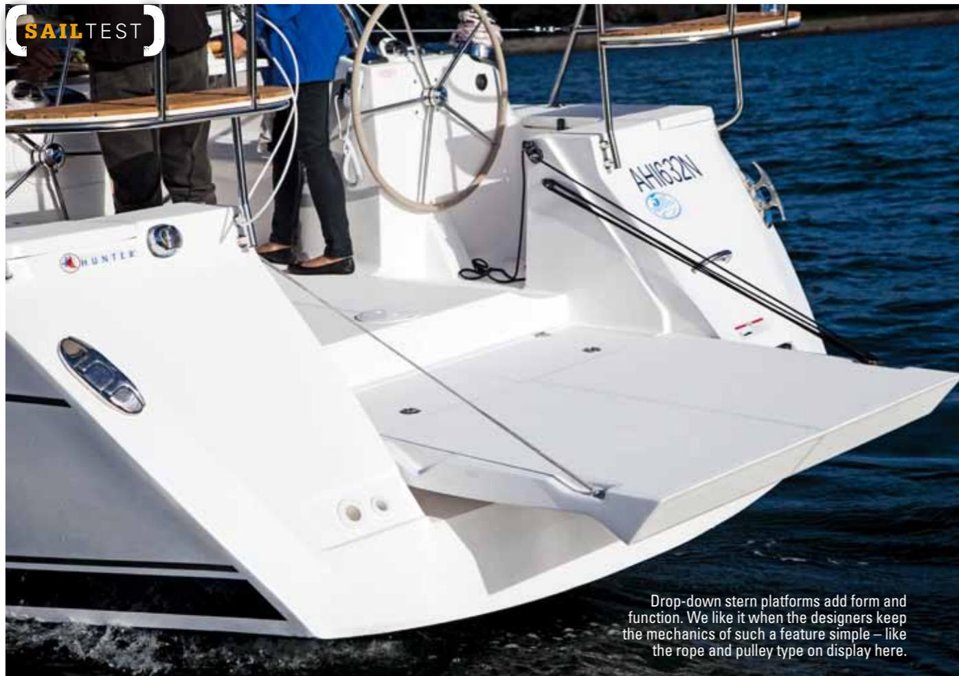
Drop-down stern platforms add form and function. We like it when the designers keep the mechanics of such a feature simple – like the rope and pulley type on display here.
