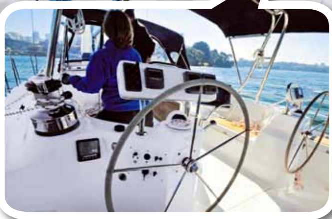
There's no shortage of shade with Hunter's cockpit targa arch (above) supporting a massive bimini, plus the traveller. Instead of separate binnacles, steering stations (left) are incorporated in the superstructure moulding.
