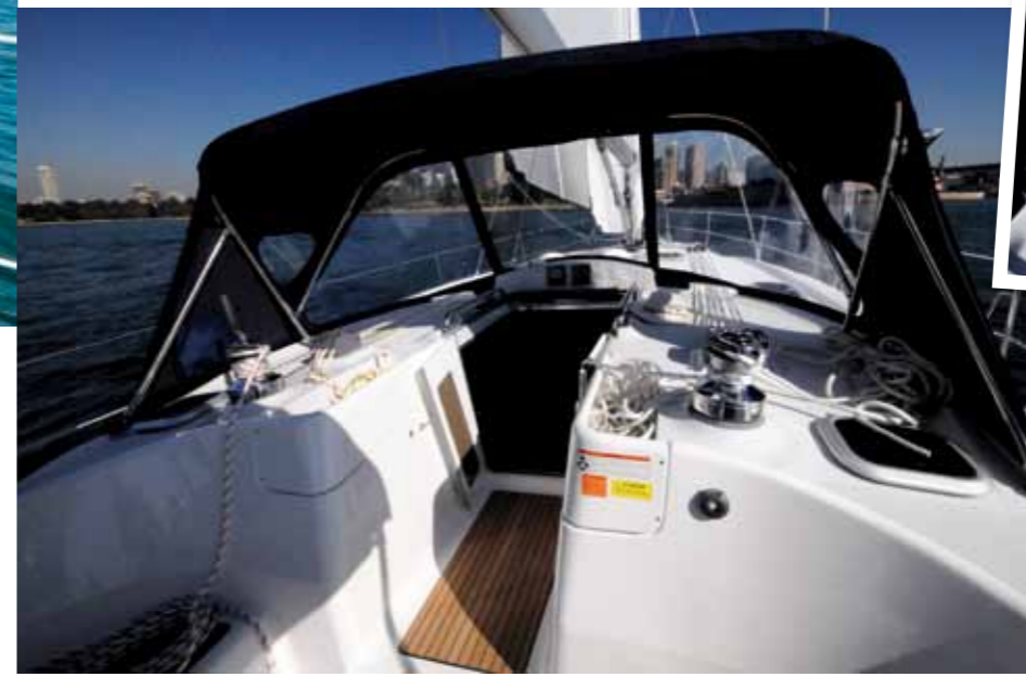
Staysail (top) is a self-tacker and the test boat had an infill to fit between the dodger (above) and bimini, enclosing the entire cockpit. Two vertical transom gates (above right) access the integrated swimplatform.
