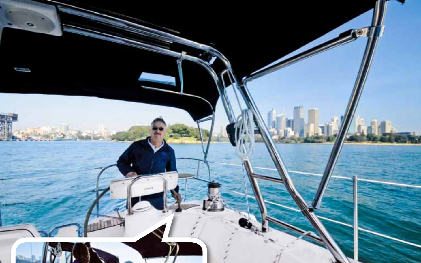
There's no shortage of shade with Hunter's cockpit targa arch (above) supporting a massive bimini, plus the traveller. Instead of separate binnacles, steering stations (left) are incorporated in the superstructure moulding.
